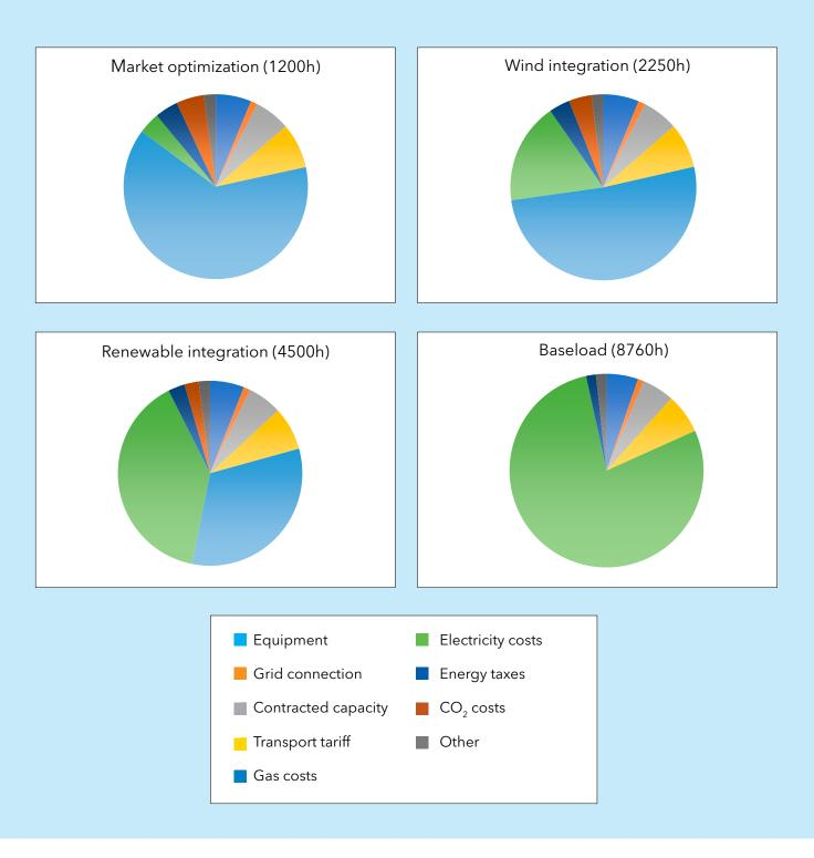
Figure 13 - Cost distribution of the hybrid boiler scenarios
