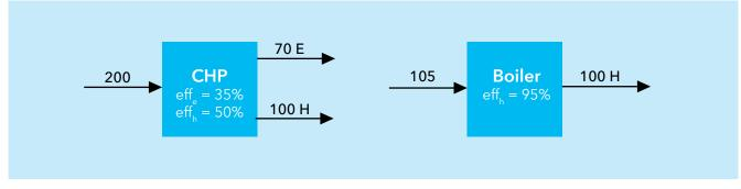
Figure 9 - Relevant energy streams when replacing a CHP-unit or a gas-fired boiler with an electric boiler
